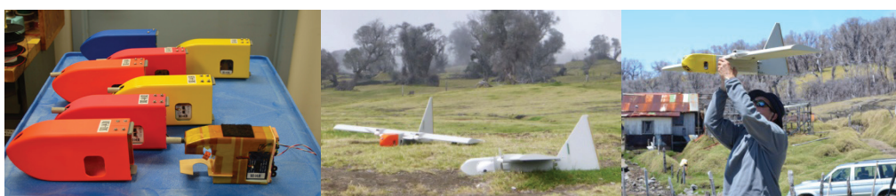
Figure 2.27: Dragon Eye UAS nose cones as designed for sulfur dioxide in situ sampling.
