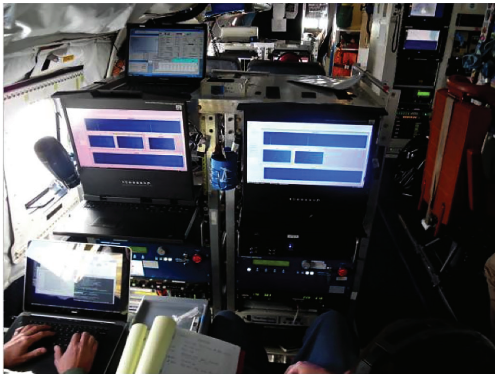
Figure 2.24: ATM Lidar workstation and data collection during IceBridge aboard the NASA DC-8.
