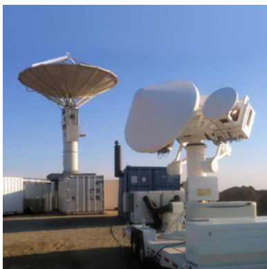
NPOL (left) is NASA's premier weather radar. It is one of only two mobile S-band dual-polarization radars.
