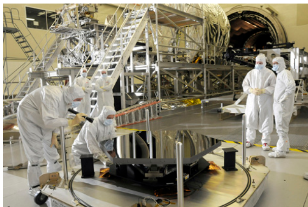
A primary mirror segment is prepared for cryogenic optical testing in the XRCF at MSFC. Credit: NASA/MSFC
