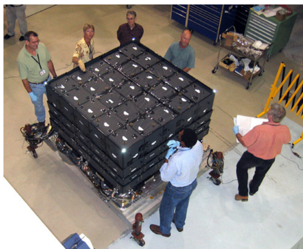
The fully assembled Fermi Anticoincidence Detector prior to thermal blanket installation. Credit: NASA/GSFC
