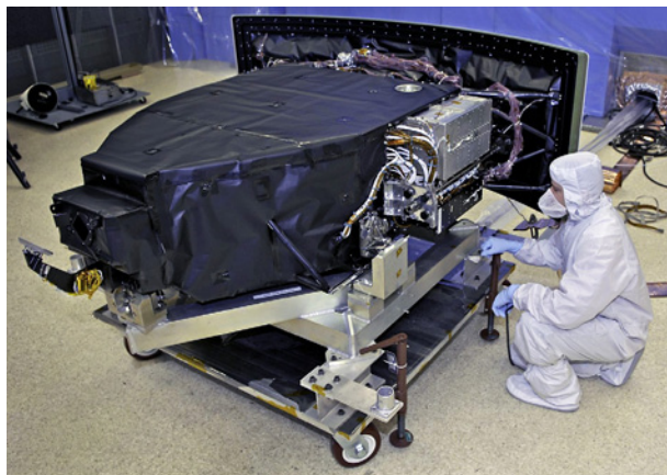
GSFC personnel completed integration of Wide Field Camera 3 in early 2008. The instrument successfully underwent a comprehensive environmental test program and now awaits launch. Credit: NASA/GSFC
