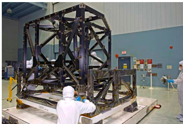
NASA engineers check out the unwrapped ISIM structure in the Goddard clean room. The ISIM Structure supports and holds four Webb telescope science instruments. NASA/Chris Gunn
