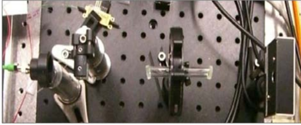
A simple iodine wavemeter based on a frequency-doubling waveguide and a fixed-pressure short iodine cell aids in heterodyne acquisition.
