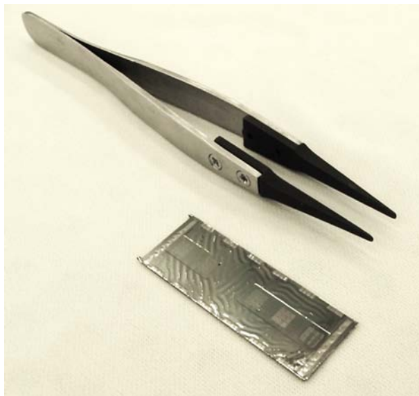
A linear-array MKID test structure fabricated by the GSFC Device Development Laboratory.
