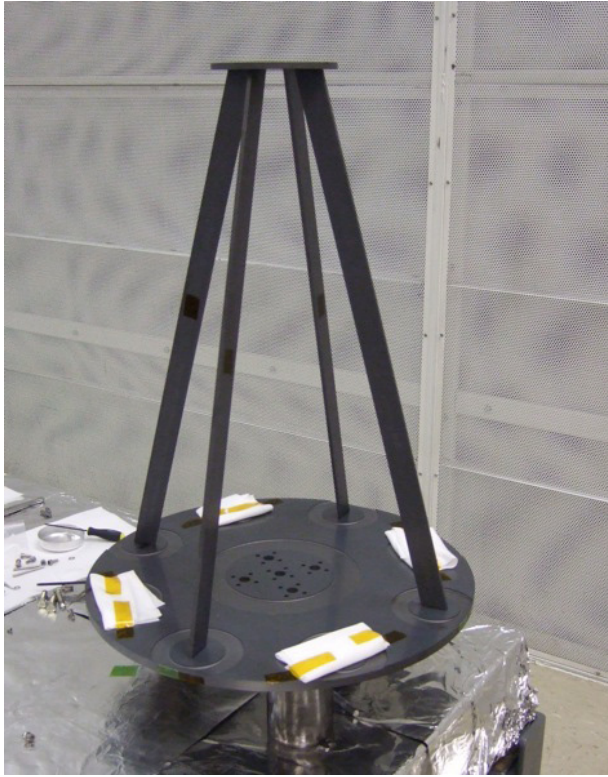
The completed silicon carbide telescope structure. A white cloth visible on the primary plate protect the optics mounting pads from scratches and dust.
