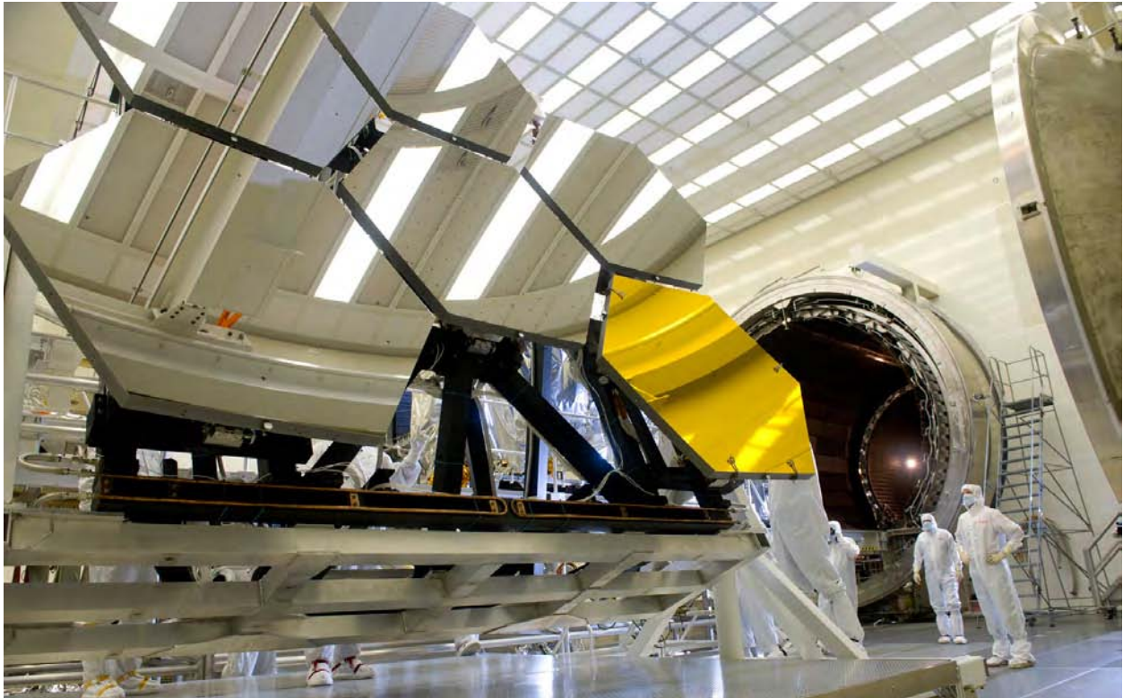
A Ball Aerospace optical technician inspects six Webb primary mirror segments—one with its gold coating—prior to cryogenic testing in the X-ray and Cryogenic Facility at NASA's Marshall Space Flight Center. Credit: NASA/MSFC/David Higginbotham
