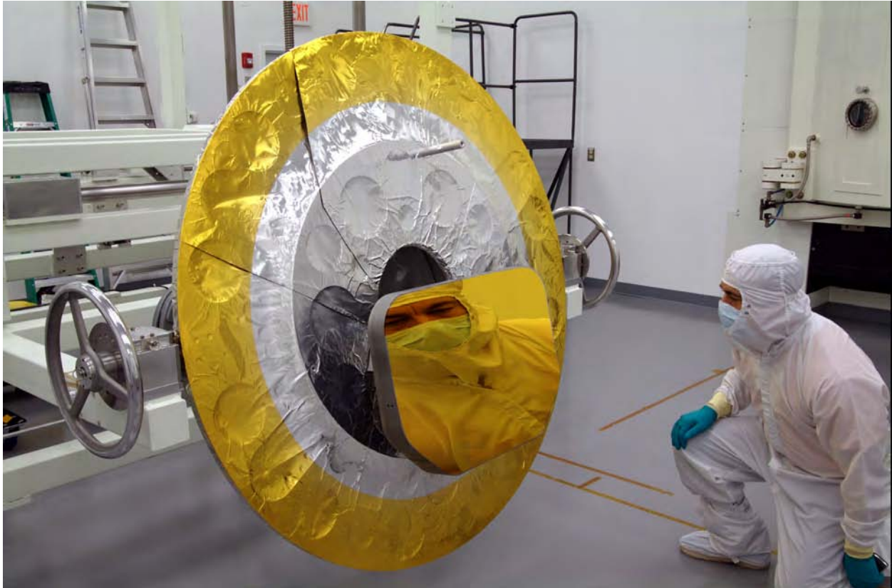
The coated flight tertiary mirror for Webb. Credit: Ben Gallagher (Ball Aerospace) and Quantum Coating Incorporated.
