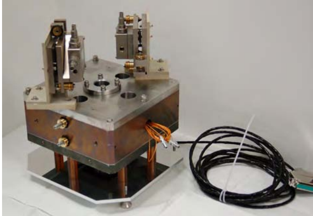
The OATM actuator test bed was used to verify that the piezo-electric inchworm actuator was capable of movement over 2 cm while maintaining position stability of better than 1\text{nm}/\text{Hz}^{1/2} in the LISA measurement band.
