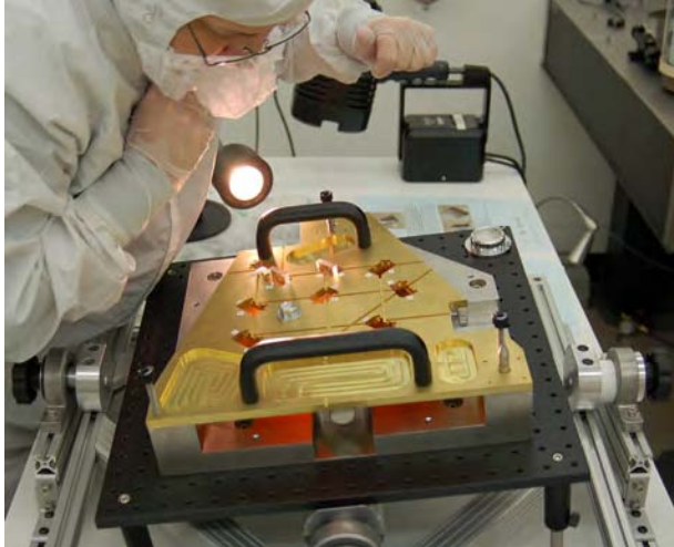
L. Miner inspects a hydroxy-catalysis bond made during construction of a prototype LISA frequency reference bench.
