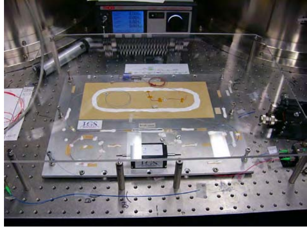
A Ytterbium fiber amplifier suitable for LISA was developed at GSFC by Numata and Camp.
