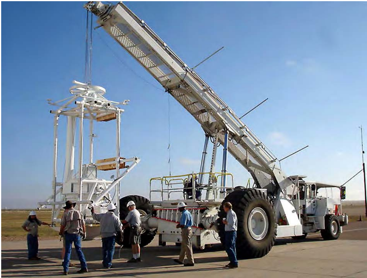
Proto-EXIST1 payload carried by the Columbia Scientific Balloon Facility launch vehicle at Ft. Sumner, N.M. prior to launch on Oct. 9, 2009. The detector array lies within the pressure vessel at the bottom of the gondola. The coded aperture mask is on the top end of the pressure vessel. The long vertical tube is the star camera. The gondola, provided by Marshall Space Flight Center, is an azimuth-over-elevation design.
