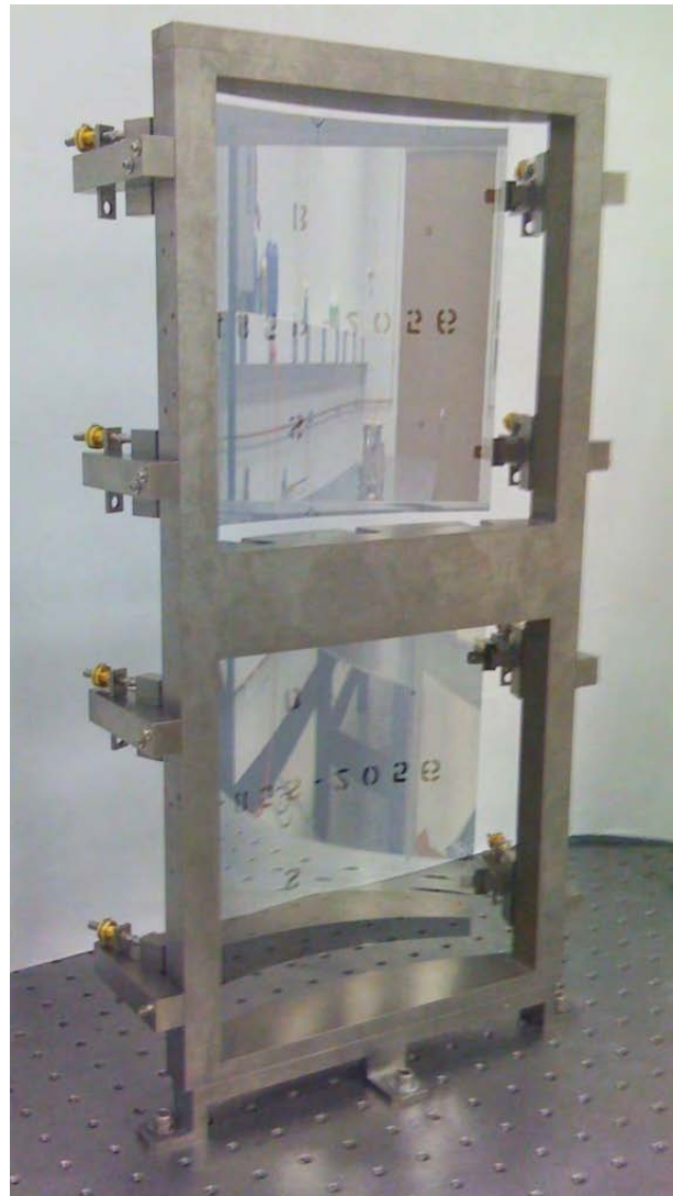
An aligned and bonded IXO mirror pair that has been X-ray tested.
