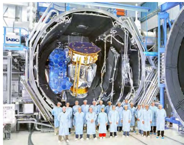
The LISA Pathfinder spacecraft (in gold foil) sits atop its propulsion module (silver foil) prior to the thermal balance test campaign.
