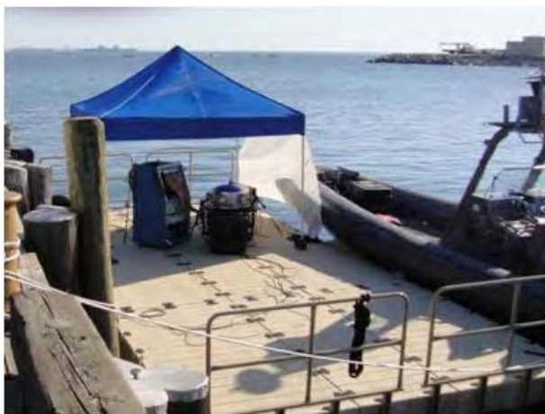
During the static over-water tests of the 30 cm NIC conducted at Fort Monroe, Va., the NIC was placed on a floating dock and the source was located in the bow of a boat, shown here moored to the dock.
