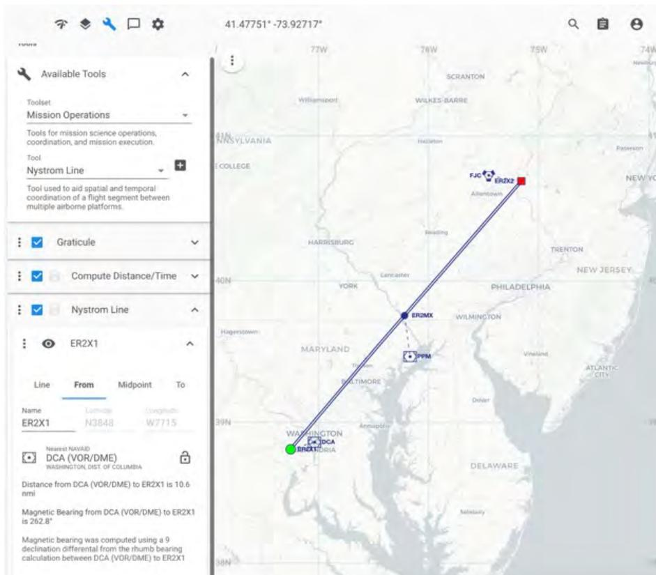
Figure 63. Screenshot showing the new Nystrom Line tool. The tool assists mission coordinators with making rapid adjustments when planning science flight segments involving multiple airborne platforms.
