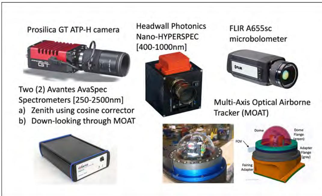
Figure 36. HYPPPOS aircraft instrumentation.
