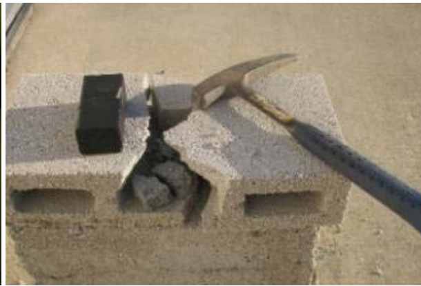
A demonstration of the impact resistance of the lunar cement was carried out for a NHK Japan TV program filmed at GSFC. The sample (black solid rod) remained intact after being smashed with a rock hammer. The supporting cinder block broke apart.
