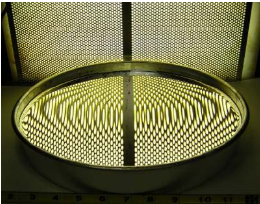
A prototype telescope mirror made using lunar cement. We conceptualize that very large mirrors and structures could be made in situ on the lunar surface.
