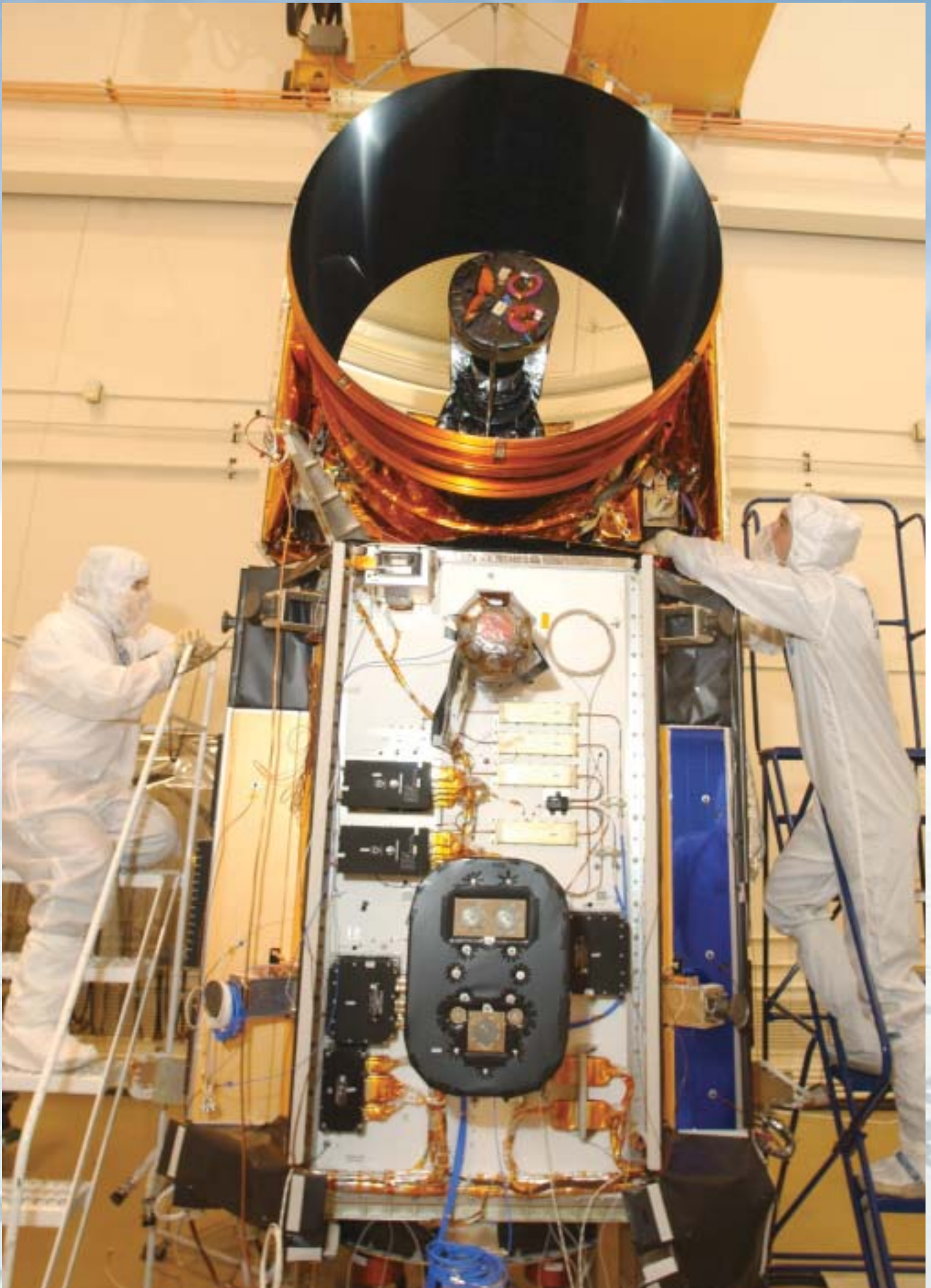
The Geoscience Laser Altimeter System (GLAS) on the Ice, Cloud, and land Elevation Satellite (ICESat) spacecraft immediately following its initial mechanical integration on June 18th, 2002. Note that ICESat's solar arrays have not yet been attached. Left – Gordon Casto, NASA/GSFC. Right – John Bishop, Mantech. Courtesy of Ball Aerospace & Technologies Corp.
