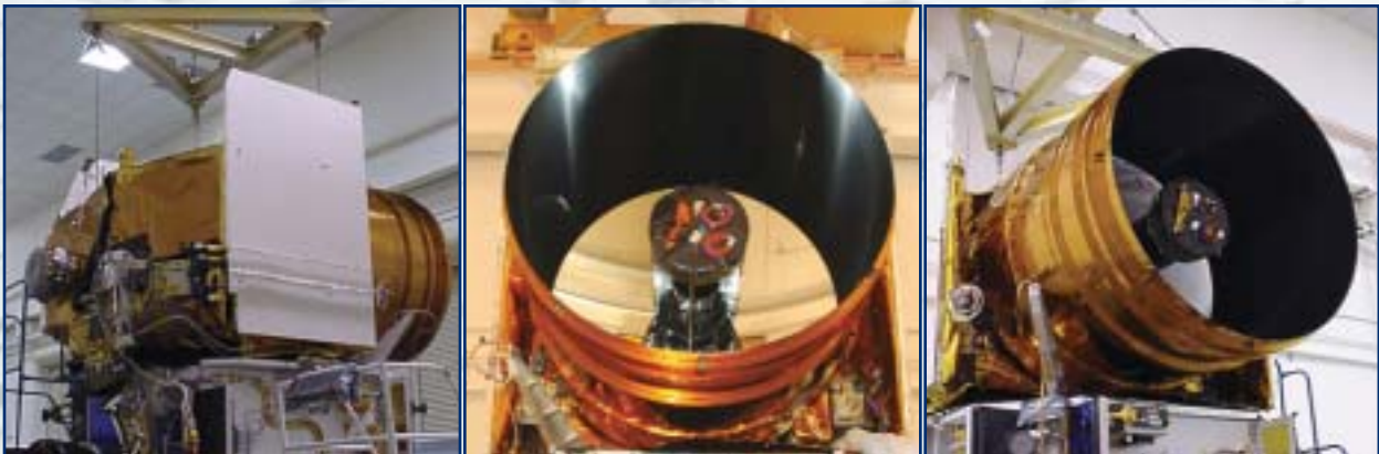
Three views of the GLAS instrument following integration with the ICESat satellite at Ball Aerospace & Technologies Corp. in Boulder, Colorado. Courtesy of Ball Aerospace.
