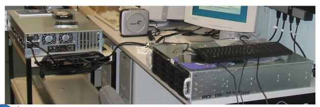
**Figure:** Two Core i7 workstations interconnected via 10 Gigabit Ethernet in test configuration prior to shipping to SC09.
