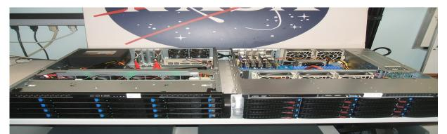
Figure: Right case houses Core i7 cores, DDR3 memory, NIC, two "internal" controllers each with eight disks and two "external" controllers; left case houses sixteen SAS-connected disks.
