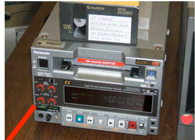
A Panasonic AJ-HD1200AP HD player, loaned from GSFC's TV Studio (courtesy of Pat Kennedy), provides one of the HD video stream sources.
