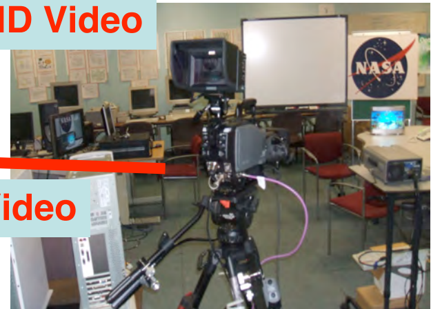
A Hitachi SK-3010P HD camera, loaned from GSFC's TV Studio (courtesy of Pat Kennedy), provides one of the realtime HD video stream sources.
